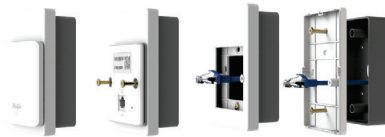
Universal Mount Kit Installation on US Junction Box (RG-AP110-L)
