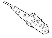
Figure 3 Dual-core LC Connector
