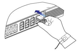
2. When you connect the SFP+ module to the optical fiber network, use the optical fiber jumper. Based on the connector type of the Interconnecting ports, choose the jumper with corresponding connectors.
