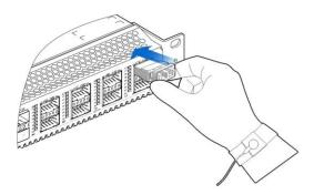
Figure 12 Installing the Pull-tab QSFP+ Module
