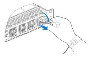
Figure 14 Schematic Diagram for Pulling out the pull-tab QSFP+ Optical Module
