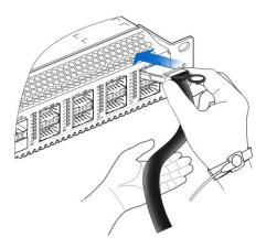
2.After installing the plug of the power cable module, connect the power cable to the Ethernet network, and the switch port indicator "LINK/ACT" will be on; otherwise, check that the connector of the power cable is correctly connected;
