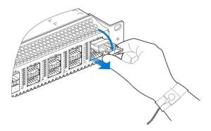
Figure 14 Schematic Diagram for Pulling out the pull-tab QSFP28 Optical Module
