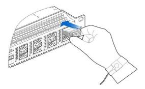
Figure 12 Installing the Pull-tab QSFP+ Module
