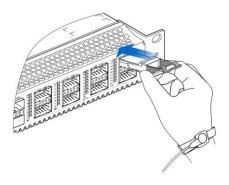
2. When you connect the 40G QSFP+ module to the optical fiber network, use the optical fiber patch cord. Based on the interface type of the Internet ports, choose the jumper with corresponding interfaces.
