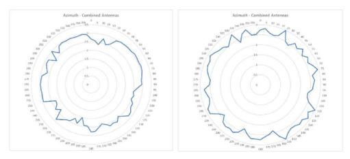
RG-AP730-L 2.4GHz (Left) and 5GHz (Right) Azimuth Antenna Patterns
