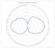
RG-AP720-L 2.4GHz (Left) and 5GHz (Right) Elevation Antenna Patterns
