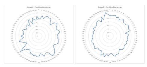
RG-AP720-L 2.4GHz (Left) and 5GHz (Right) Azimuth Antenna Patterns
