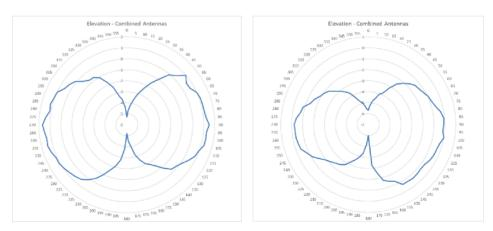
RG-AP730-L 2.4GHz (Left) and 5GHz (Right) Elevation Antenna Patterns
