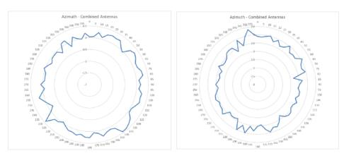
RG-AP710 2.4GHz (Left) and 5GHz (Right) Azimuth Antenna Patterns
